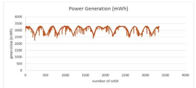
Fig. 2. CubeSat power generation analysis during six months period of time (simulated by STK)
