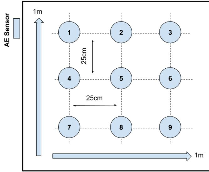
Fig. 2. Location of PDs relative to AE sensor [5]
