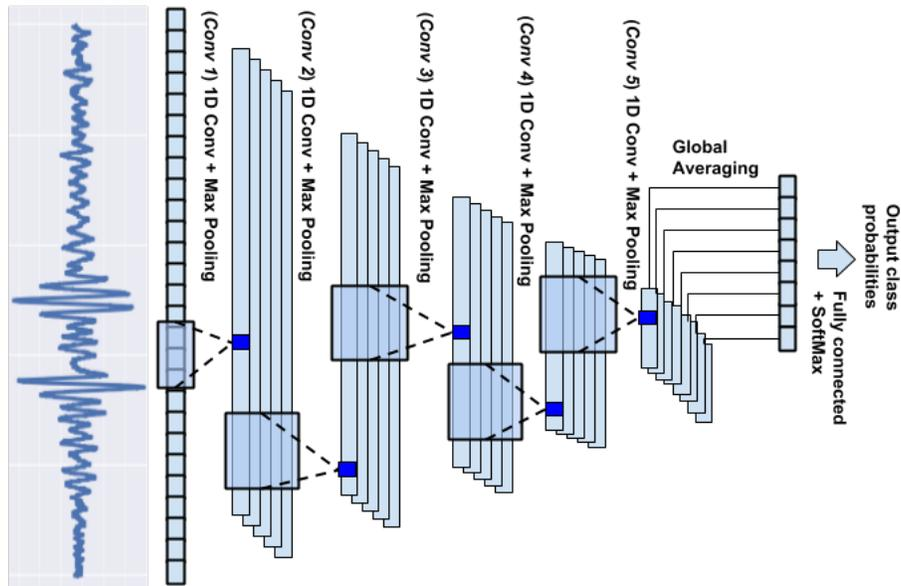
Fig. 1. 1D-CNN - Model architecture
